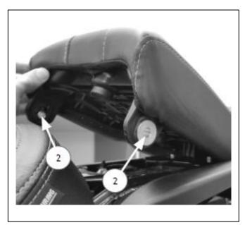
**3** Remove the two bolts (3) and sleeves (4) securing the rider seat to the chassis. Retain the bolts and sleeves for reuse. Lift the rider's seat from the rear and pull rearwards to remove it.
